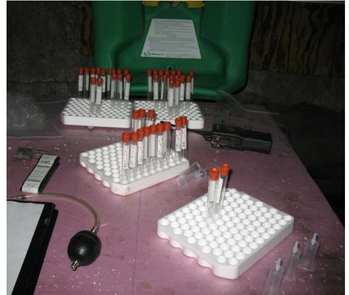
Figure 4. Vacutainers used to collect SF 6 concentration samples inside and outside of the RA.
