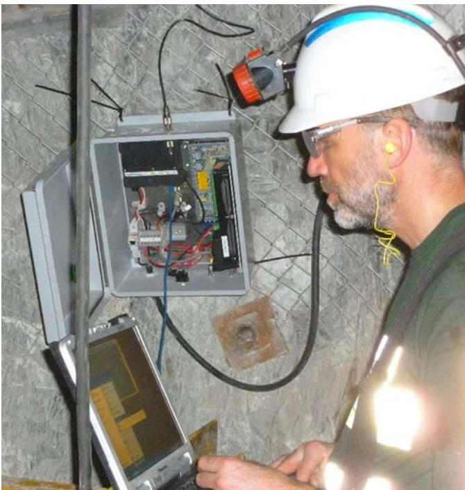
Figure 5. Evaluating wireless link performance.
