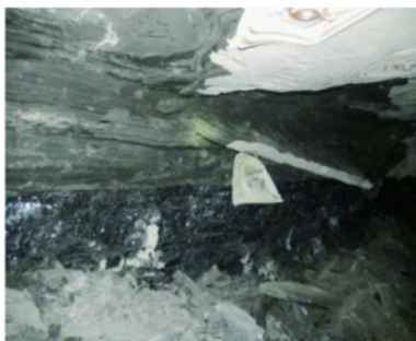
Fig. 19. Rib sloughage at the panel side in the bleeder entry of Panel II in the lower seam.
