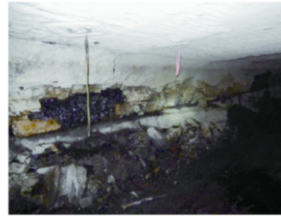
Fig. 15. Rib sloughage outby the pillaring line during retreating in the upper seam.
