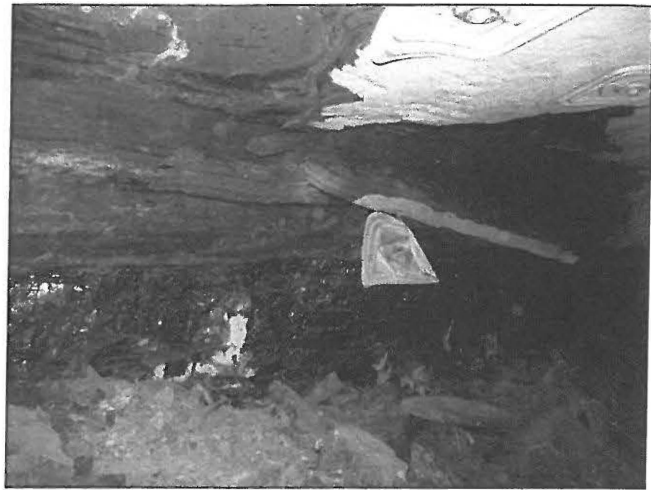
Figure 19. Rib sloughage at the panel side in the bleeder entry of panel II in the lower seam.
