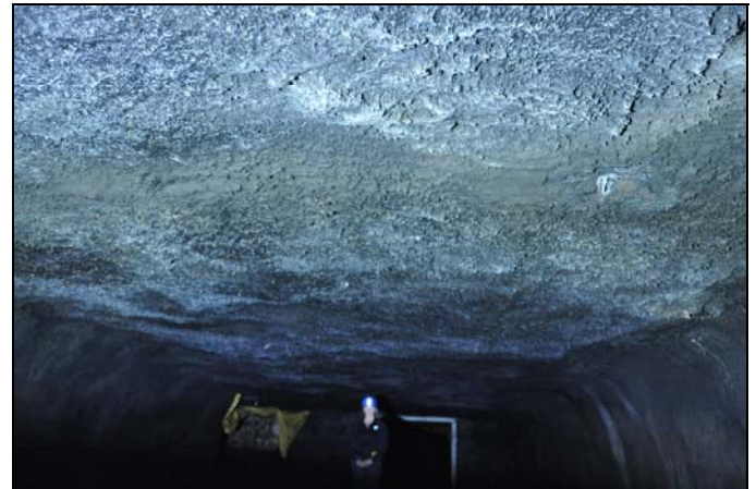
Figure 5. Illumination provided by prototype LED area light for visual inspection of refuge alternative sites. The illumination can also be directed to illuminate the floor area. The distance to the person pictured is about 9.1m (30 ft).
