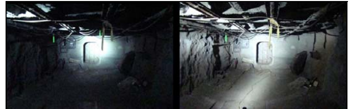
Figure 4. Illumination from a traditional LED cap lamp (left) and from the NIOSH LED cap lamp (right).
