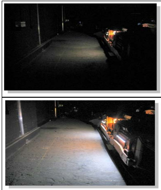
Figure 1. A CMM with standard lighting (top) compared to with NIOSH LED lighting (bottom).
