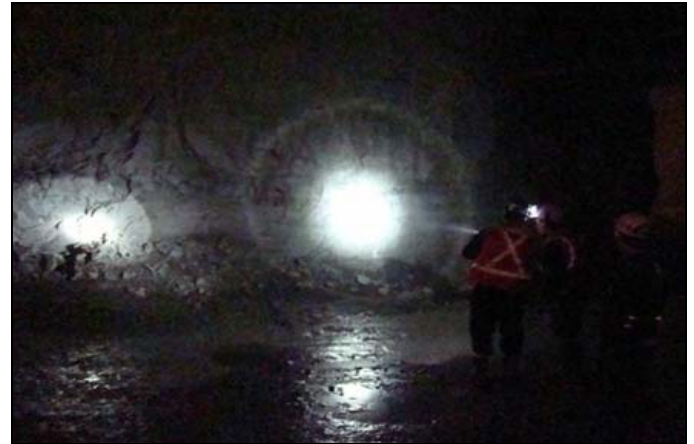
Figure 3. Comparison of spot beam intensity between a cordless LED cap lamp (left) and the NIOSH metal/nonmetal LED cap lamp (right).
