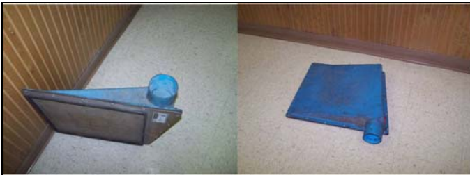
Figure 3. Original square air curtain design, by Donaldson Company, Inc.
