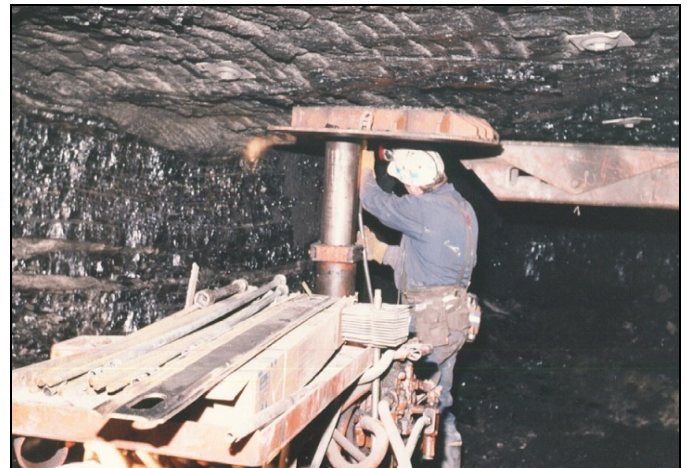
Figure 1. Roof bolter operator under roof canopy during roof drilling.
