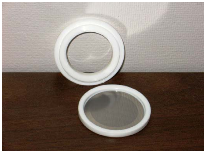
Figure 2. The open-faced cassette used with the 1500-pDR. The 37-mm filter is placed on the stainless steel backing and the upright ring is pressed onto the filter.
