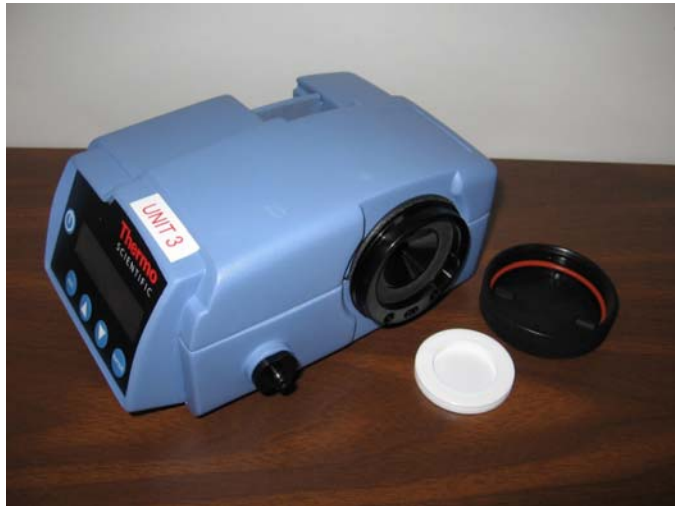
Figure 1. The 1500-pDR showing the open-faced filter cassette and the location where the filter cassette is attached to the sampling unit.
