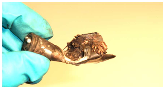
Fig. 2. Ruptured LG Chem cell crushed by the plastic wedge that ignited 6.5% \text{CH}_4 -air.
