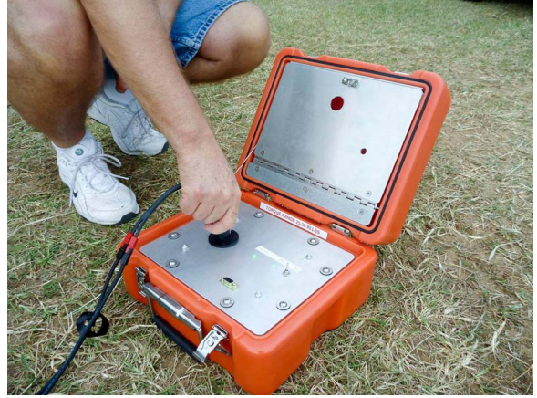
Fig. 3. E-Spectrum subsurface transceiver shown on surface.
