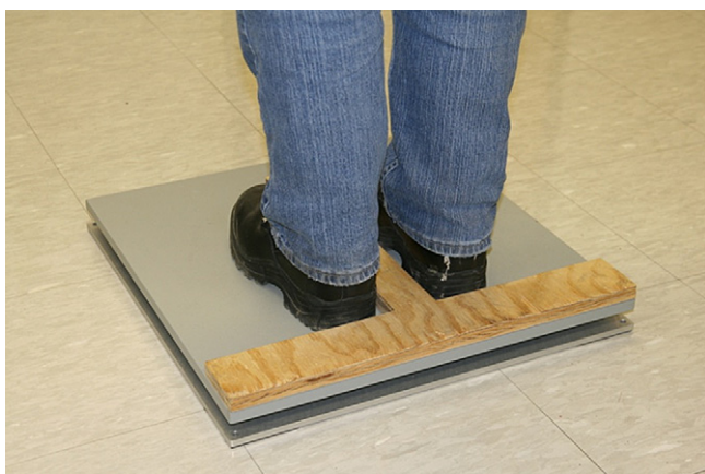
Fig. 5. Force plate showing placement of the feet and T-shaped separator.
