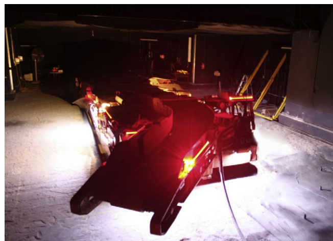
Fig. 2. The visual warning system installed on a continuous mining machine. The red warning light indicates that the conveyor is going to swing to the right. (For interpretation of the references to color in this figure legend, the reader is referred to the web version of this article.)
