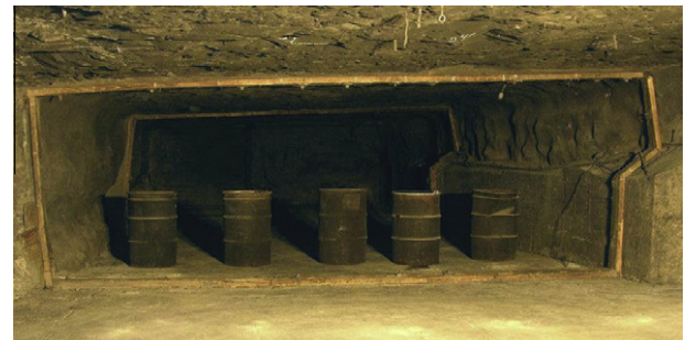
Fig. 3. Ignition chamber located at the end of C-Drift. (Figs. 3–5 were provided by Eric Weiss of NIOSH, Office of Mine Safety and Health Research's then Disaster Prevention and Response Branch.)
