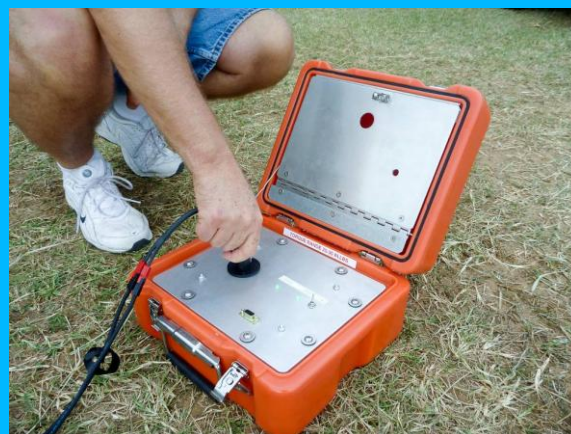
Fig. 3. E-Spectrum subsurface transceiver shown on surface
