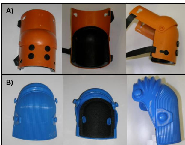
Figure 2: Kneepads used in this study. Outer shell, inner padding, and side views of the articulated kneepad (A) and the non-articulated kneepad (B). Both kneepads used straps that attached a little above and below the crease of the knee.
