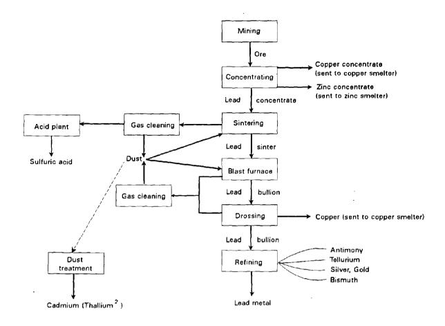
Figure 9.—Lead processing schematic.1
