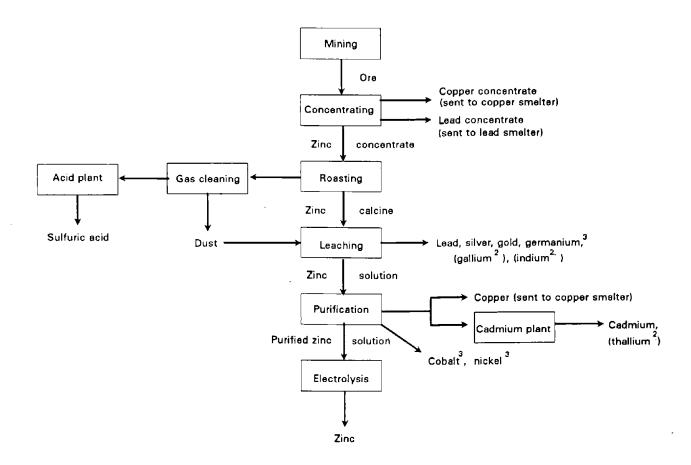
Figure 10.—Electrolytic zinc processing schematic.1
