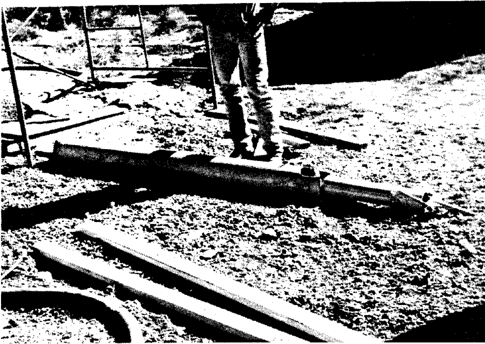
FIGURE 6. - Air jet footpiece lying on ground in extended position utilized when placing element into borehole. Footpiece barrel on right.
