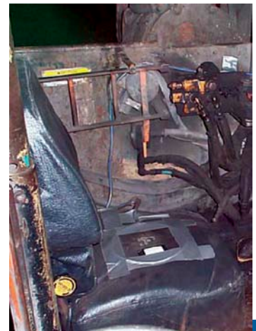
Photo 3 (a, top): Existing design for mid-seam shuttle car seat; and (b, bottom) NIOSH's experimental design.
