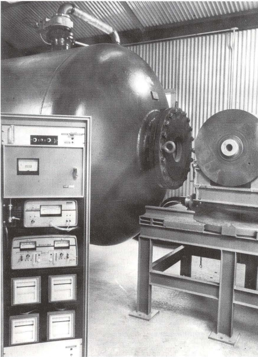
Figure 28.2 - Large Chamber used for determining the toxic fumes produced by permissible explosives. (Courtesy: R. Mainiero)
