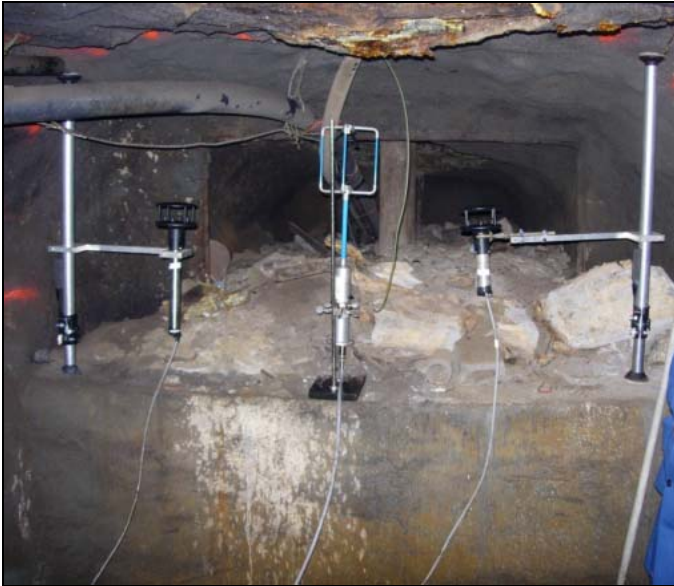
Figure 7. Test Set-up at Location 3 with the 2-axis Instruments at Low Position.
