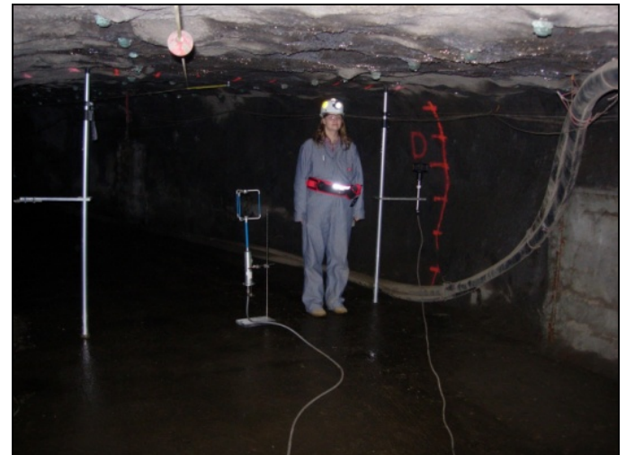
Figure 3. Stationary Obstruction 1 between 2-axis and 3-axis Ultrasonic Anemometers in Location 2.
