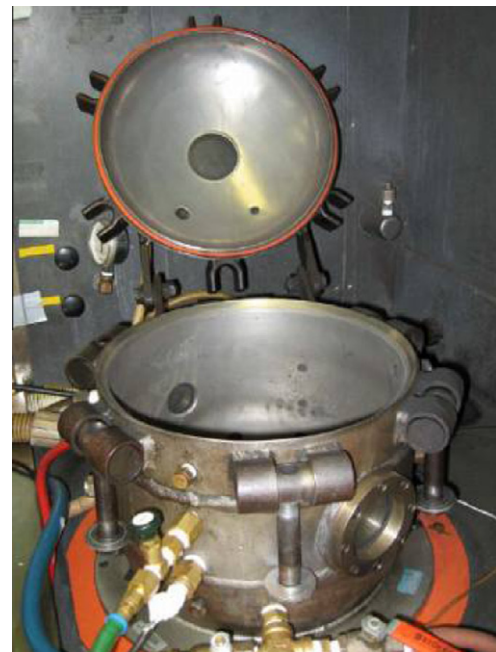
Fig. 2. The 20-L ignition apparatus.
