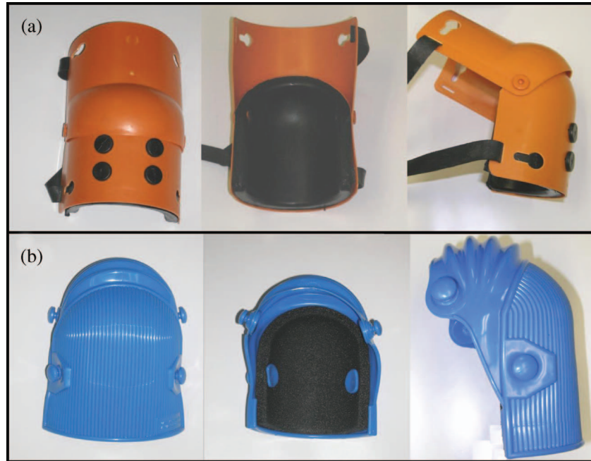
Figure 1. Kneepads used in the study: (a) articulated kneepad with hard contoured outer shell; (b) non-articulated kneepad with soft outer shell.
