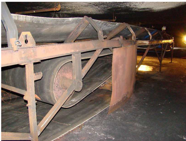
Figure 2 — 208-L (55-gal) drum as drive roller.
