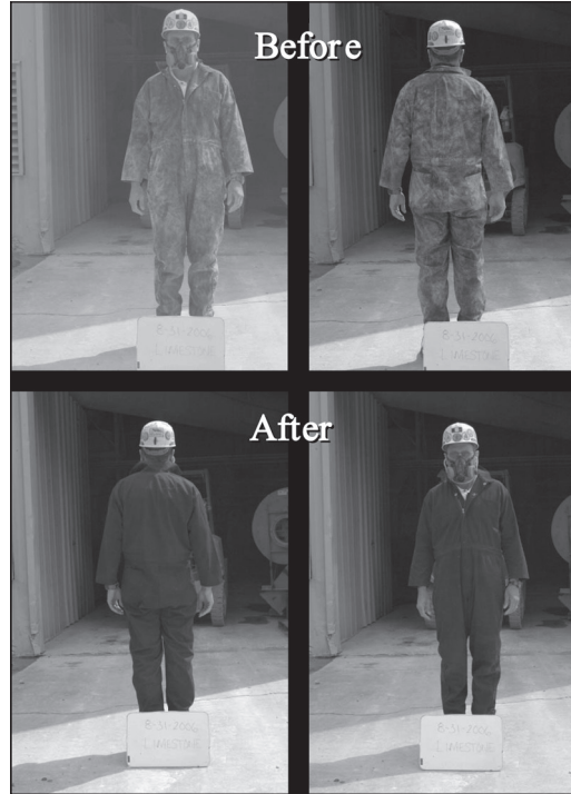
Figure 7. Test subject wearing polyester/cotton blend coveralls before and after using clothes cleaning booth
