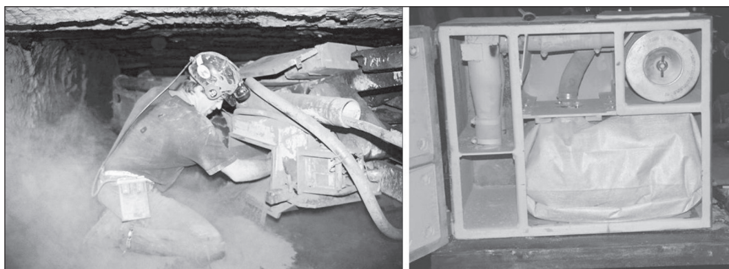
Figure 6. Miner cleaning dust collector box (left) and retrofitted collector bag filled with dust (right)
