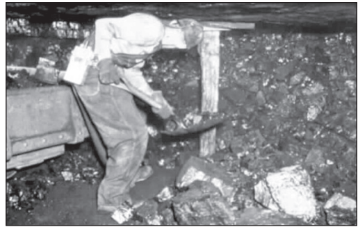
Figure 4. Hand loading with a safety post
