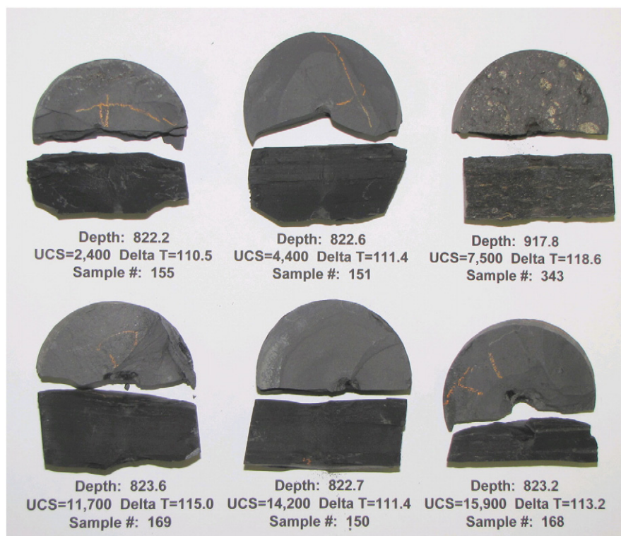
Fig. 13. Carbonaceous shale samples from corehole Kentucky A. The samples have been tested and the halves oriented to show a top view and a view of the failure surface. All samples are from the Anna shale, except the top right sample, which is from the Turner Mine shale. The samples were chosen to illustrate the wide range of UCS values observed in the carbonaceous shales, despite a narrow range of logged travel times. Depths in feet, UCS in psi and Delta T in µs/ft.
