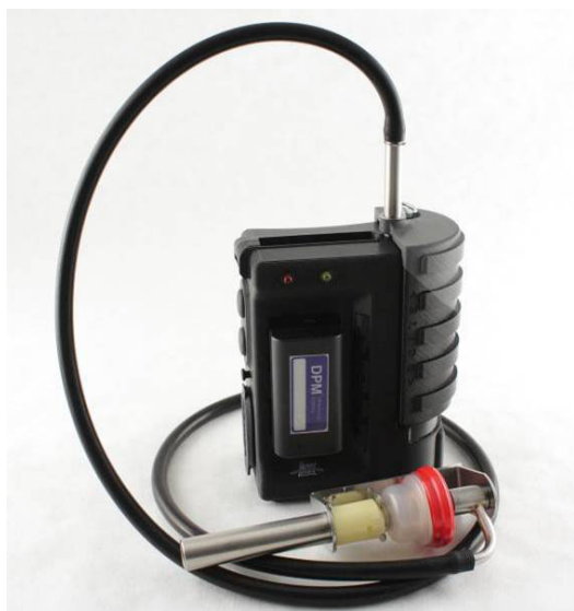
Figure 1 A photograph of the ICx DPM Monitor beta prototype showing the instrument, sampling line and size selector.
