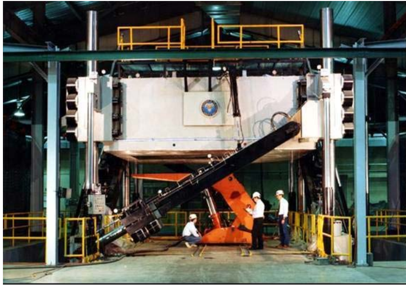
Figure 3 – NIOSH's Mine Roof Simulator (MRS) [17].
