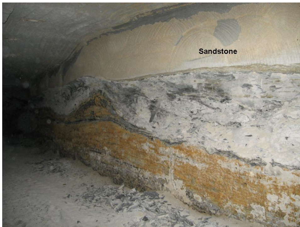
Figure 36: Sandstone layer is the roof bolt anchorage when close to the coalbed.
