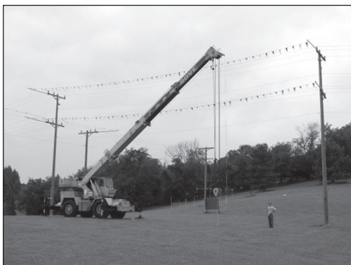
Figure 8. Full scale power line proximity alarm test at Pittsburgh Research Laboratory
