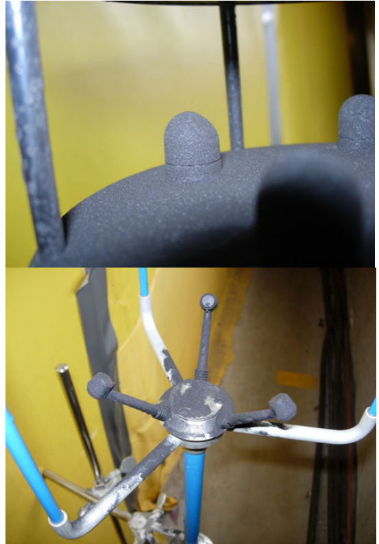
Figure 6 Wetted coal dust on 2-axis and 3-axis ultrasonic anemometer heads
