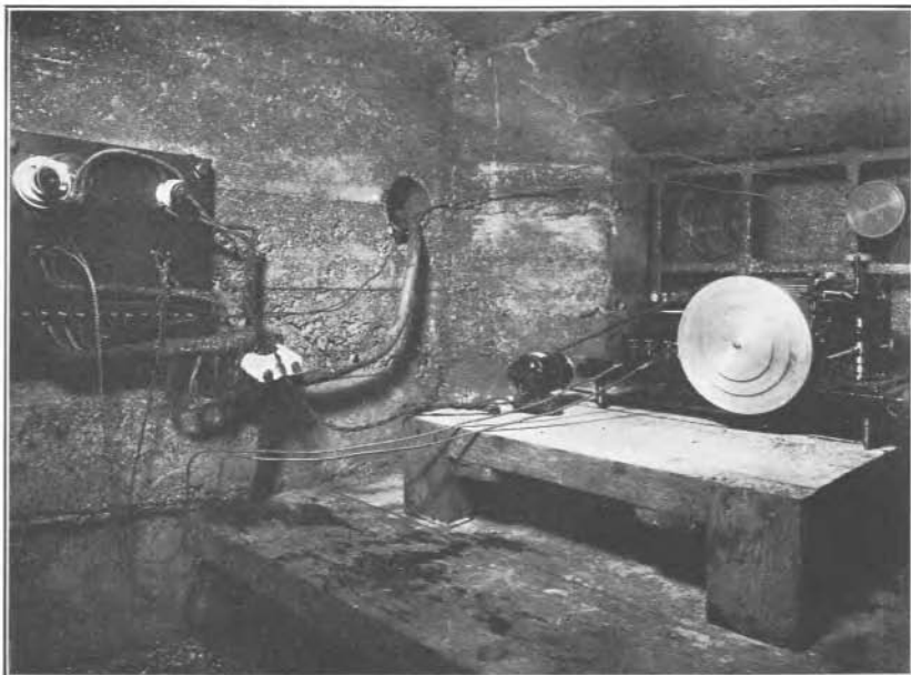
A. INTERIOR OF AN INSTRUMENT STATION, SHOWING MANOMETER AND PRESSURE CIRCUIT BREAKER.
