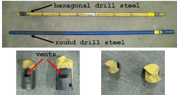
Fig. 1 – Hex and round drill steels for a 35-mm diameter drill bit (upper) and two examples of drill bits – 25 mm and 35 mm (lower).
