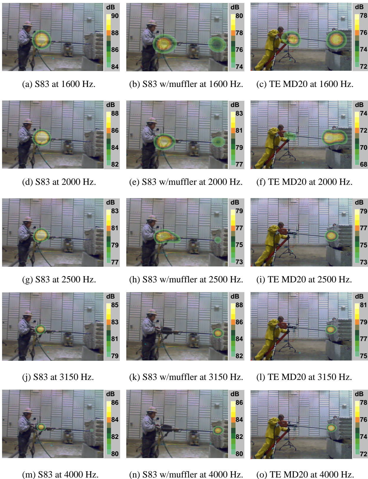
Fig. 4 - One-third octave band acoustic maps for two pneumatic drills (S83 and S83 with muffler), and an electric drill (TE MD20).
