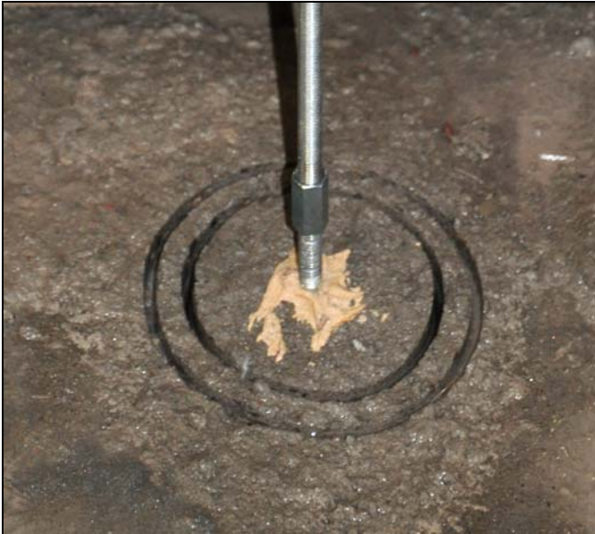
Figure 15. Parallel and concentric drill holes with extension rod connected to epoxied stud.
