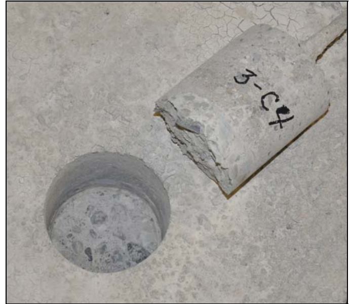
Figure 16. Adhesion test specimen showing a tensile failure surface located predominantly in the concrete substrate.
