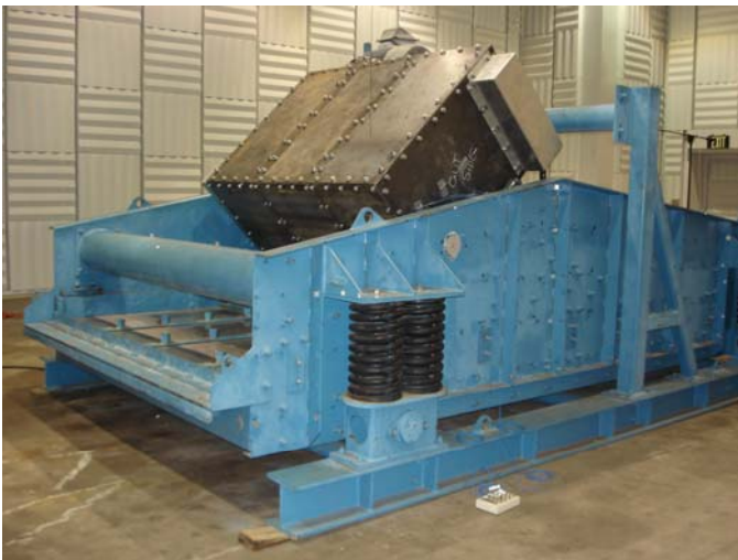
Figure 8. Second enclosure installed on vibrating screen.
