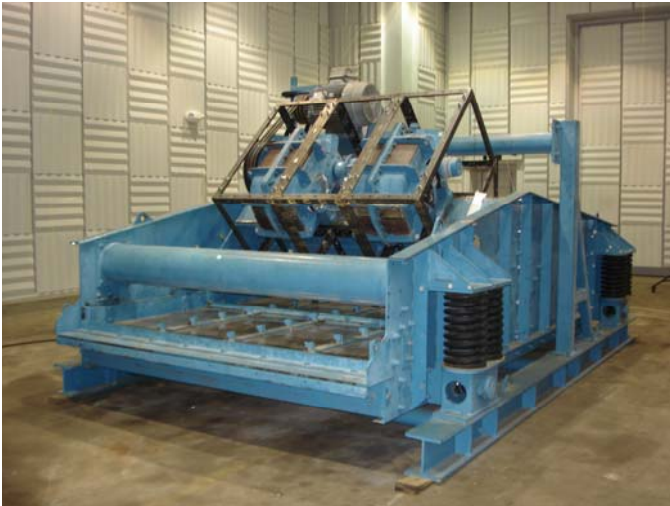
Figure 7. Steel frame for the second enclosure installed on vibrating screen.
