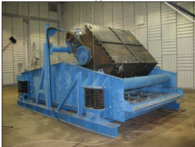
Figure 4. First enclosure constructed using a three-piece design. (a) Model showing internal duct structure and (b) enclosure installed on the vibrating screen.
