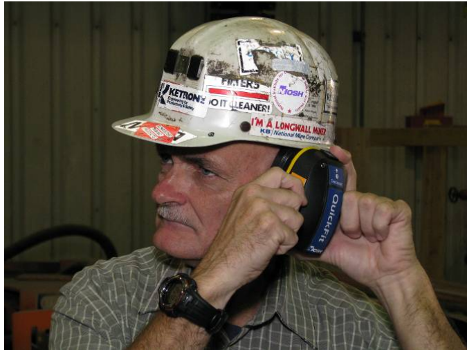
Figure 3. Worker adjusting the volume control on the QuickFit device to set his hearing threshold prior to inserting an earplug.
