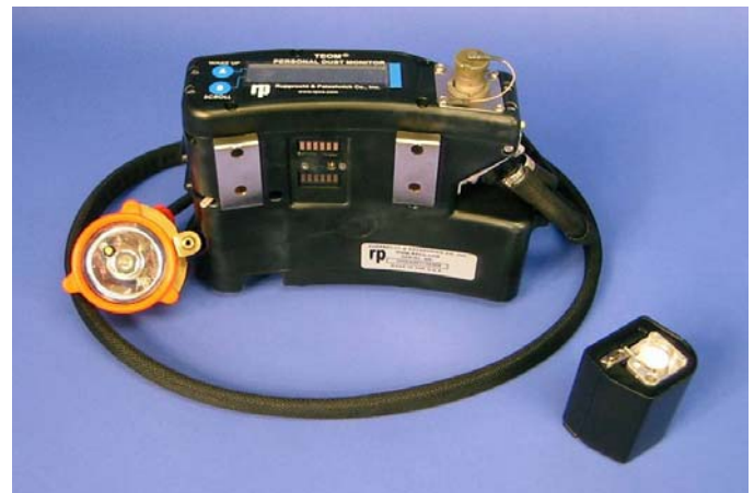
Figure 3b. Personal Dust Monitor.
