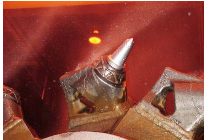
Figure 1a. Wet head bit block showing water spray behind the bit.
