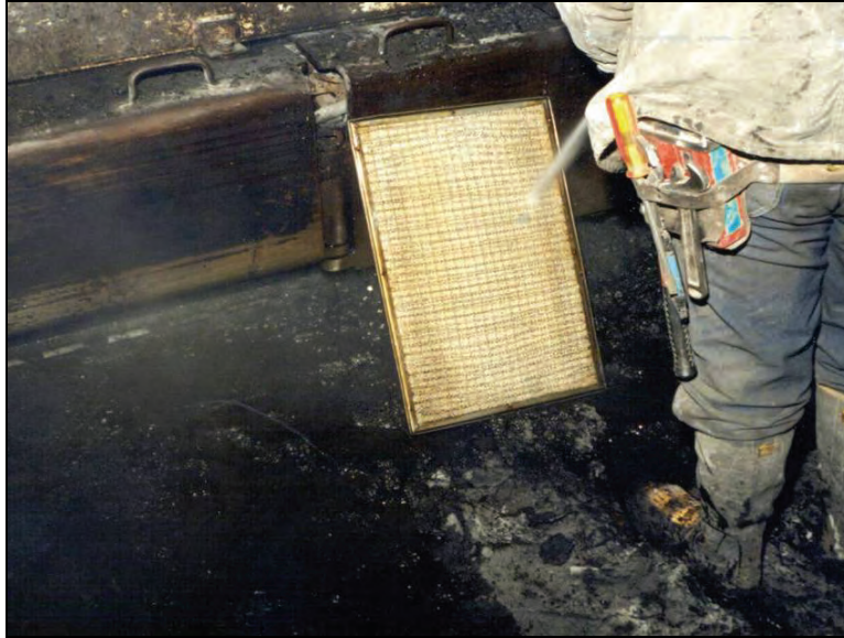
Figure 4-7.—Cleaning scrubber filter panel with water spray.
