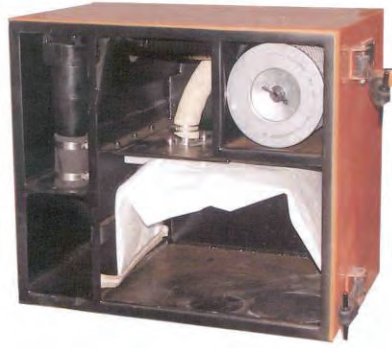
Figure 4-14.—Dust collector box with collector bag installed.
