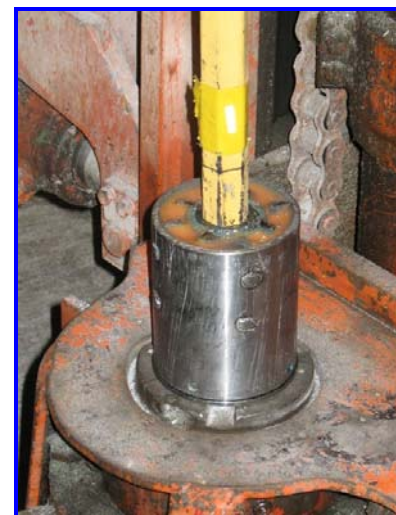
Figure 17 - Chuck isolator 2, 45 Shore A polyurethane filled
