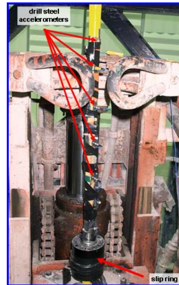
Figure 3 - Drill steel accelerometers and slip-ring assembly
