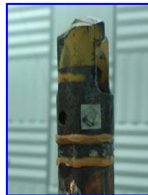
Figure 10 – Bit isolator with 60 Shore D urethane coating
