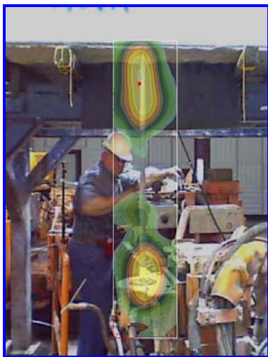
Figure 8 - Beamforming of baseline drilling, 100 dBA @ the operators' position
