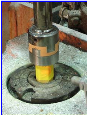
Figure 5 - Jaw-type coupling with 58 Shore D urethane spider
