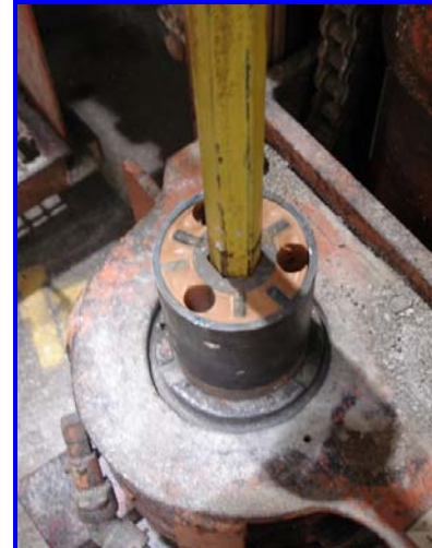
Figure 15 - Chuck isolator 1, 58 Shore D polyurethane filled
