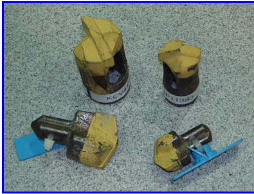
Figure 2 - Drills bits; vacuum (top), wet (bottom), 2.54 and 3.49 cm
