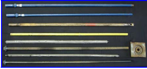
Figure 1 - Drill steels (round & hex), bolt plate, resin and resin type roof bolts, shown for 2.54 and 3.49 cm bit drilling and bolting
