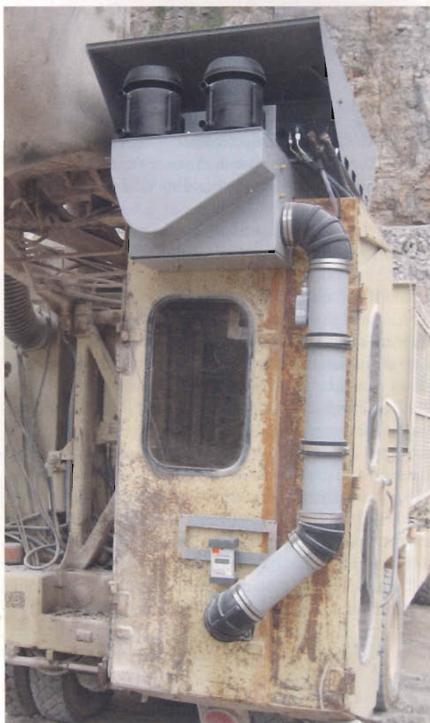
The installation of a unidirectional filtration system can greatly reduce a worker's exposure to harmful dust.
