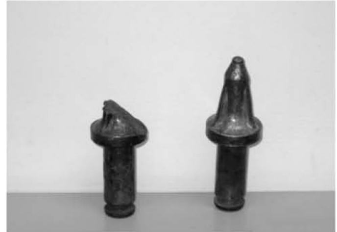
Figure 5. Comparison of worn miner bit to a new bit.
