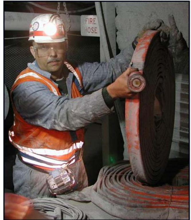
Figure 12. Typical fire hose in an underground coal mine.
