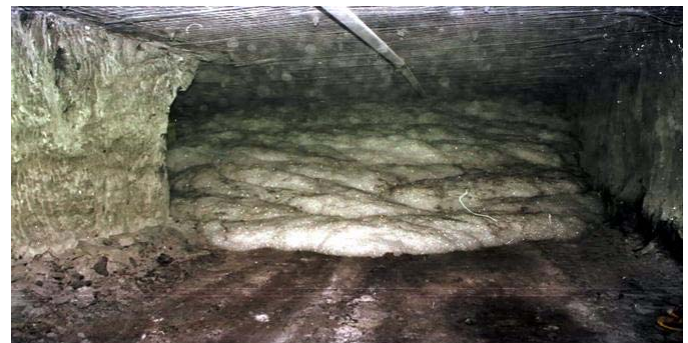
Figure 6. Leading edge of foam plug in No. 3 entry, first crosscut on left.
