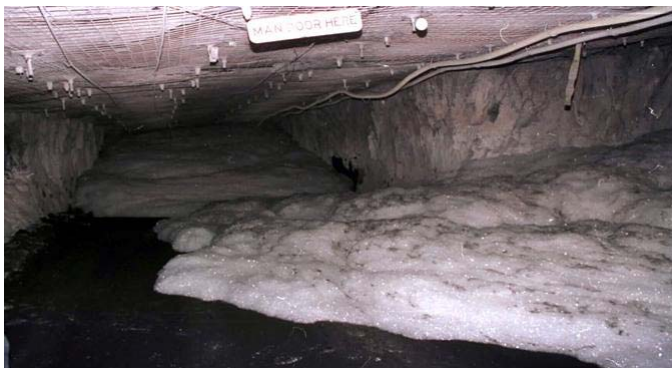
Figure 9. Leading edges of foam plug in entry No. 2 and from crosscut on right.
