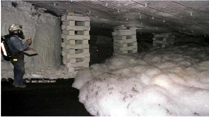
Figure 7. Foam plug in No. 2 entry.
