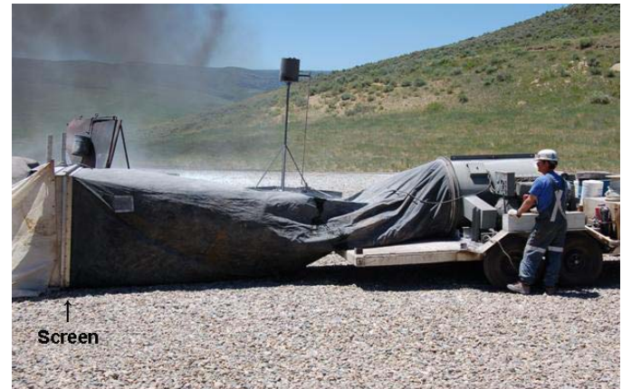
Figure 1. Jamison 18,000 cfm high-expansion foam generator with attached expandable shroud and screen.
