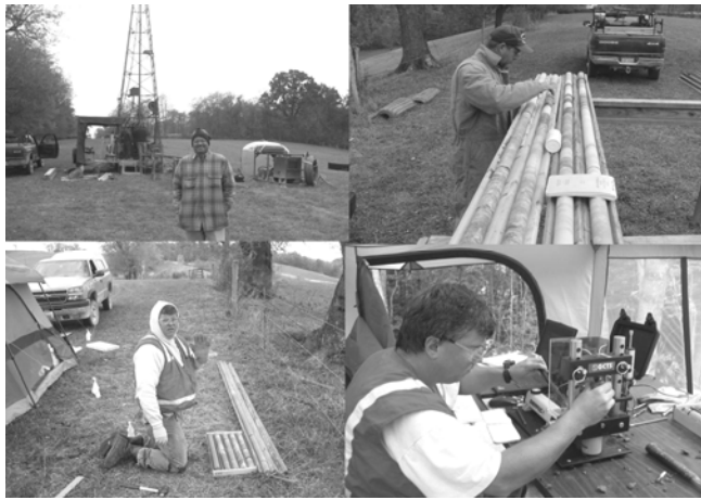
Figure 4. Pictorial overview of stages of fieldwork at both drill sites; clockwise from top left: (a) Diamond rock core drilling at site 2; (b) geologic logging of core runs at site 2; (c) axial PLT-UCS measurements of core specimen at site 1; f core runs at site 2, (d) boxing of core runs in labeled core boxed made of wax permeated cardboard at site 2.
