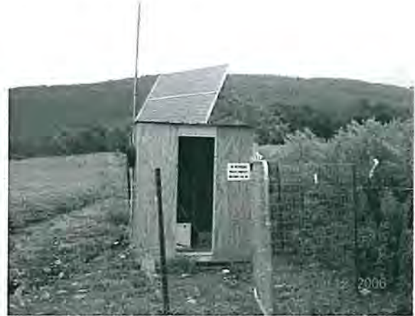
Figure 2. Microseismic data acquisition station at a borehole site.
