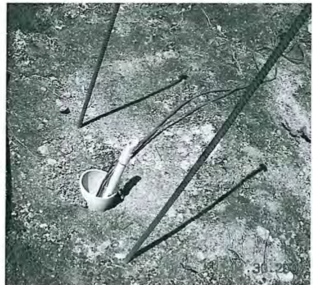
Figure 3. Cables leading from the geophones to the data acquisition processor.
