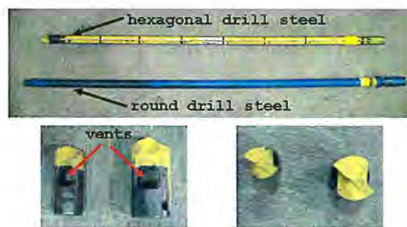
Figure 5: Hex and round drill steels for a 3.49 cm diameter drill bit (upper) and two examples of drill bits (lower).
