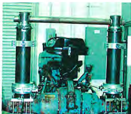
Photo 3: Second-generation AutoROPS on Ford 4600 in lab.
