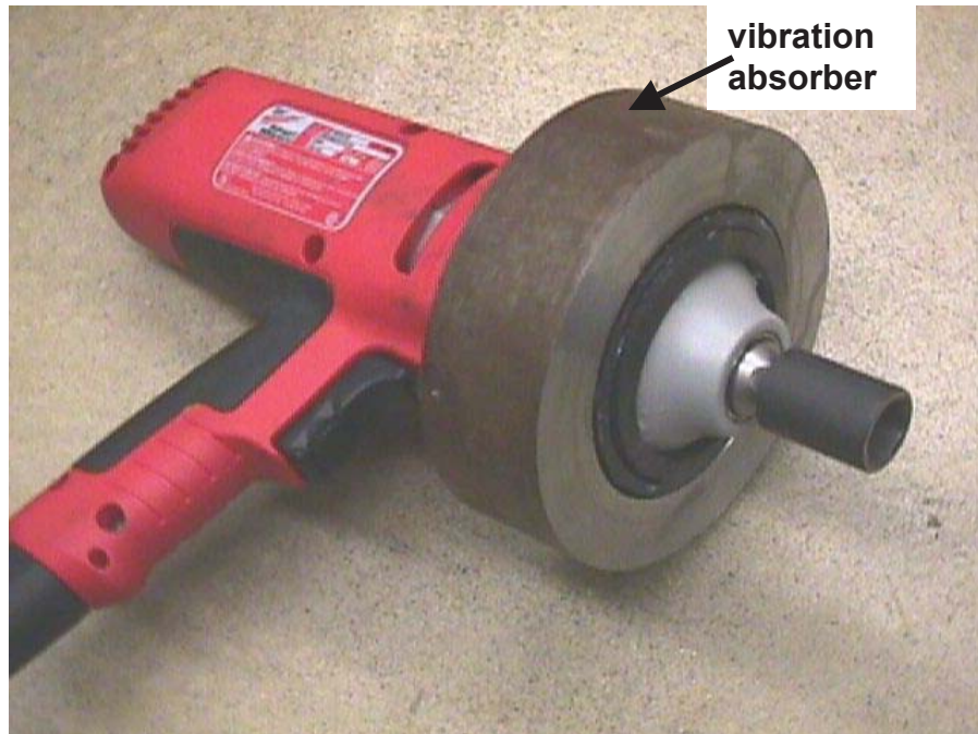
Figure 3: Impact wrench with torsional vibration absorber.
