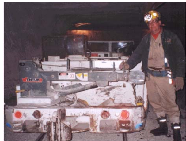
Figure 8.— Swing boom arm attached to mine vehicle.
