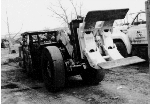
Figure 6.— Attachment used to pick up and maneuver can cribs.
