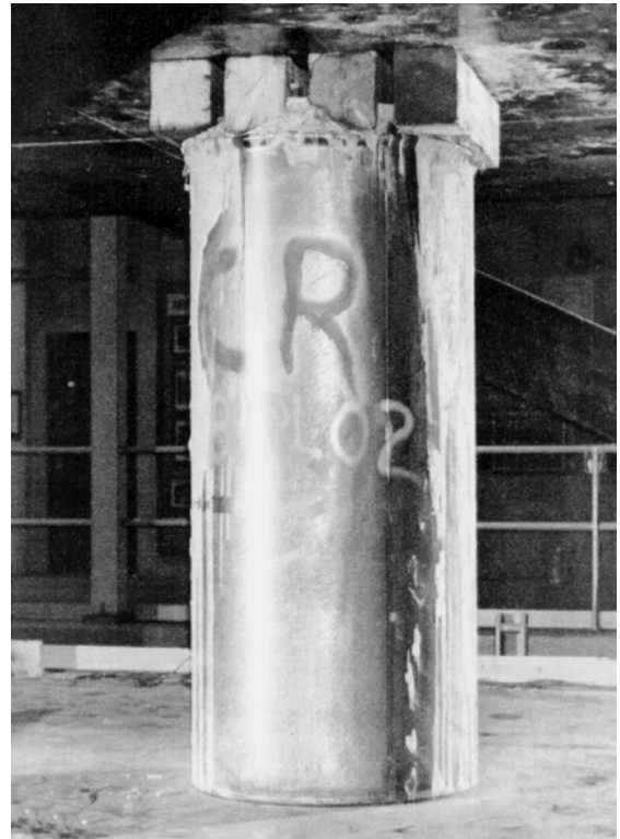
Figure 5.- Can crib used to replace wood crib in underground coal mines.
